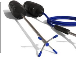
The Vectrino consists of two basic elements: the probe attached to a clyndrical housing and the processor inside the housing. From here the processed data is sent over a serial line or analog signals can be sent to an A/D converter.
