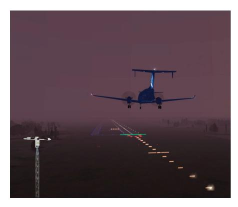
The Visibility and Present Weather Sensors GEO-SWS-100/200 have been designed for continuous environmental monitoring of roads and tunnels for traffic safety, sea ports and airports, as well as for many other classical uses in meteorology, climatology and weather networks.
