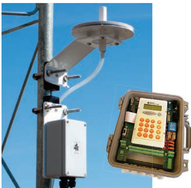
Weatherproof Enclosure and Pressure Port and Datalogger
