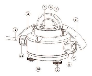
**Figure 2 GEO-SR11 overview:** (1) cable, (2) opening for fixation of sun screen, (3) thermal sensor with black coating, (4) outer dome, (5) inner dome, (6) sun screen, (7) humidity indicator, (8) dissecant holder, (9) levelling feet, (10) bubble level, (11) cable gland
